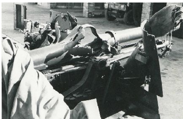
Damage From Premature
